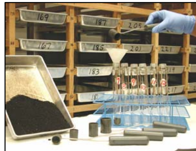
5. Scooping a pre-set volume of soil for extraction
