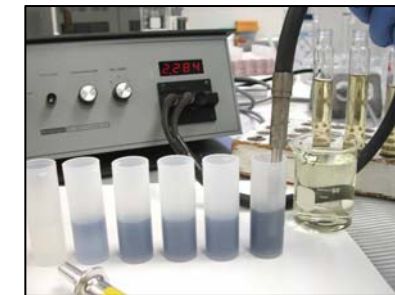
9. Measuring soil-P (blue intensity) with a probe colorimeter
