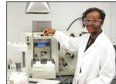
10. Measuring soil-K, Ca, Mg, and Na with the Varian atomic absorption (AA) spectrophotometer.
