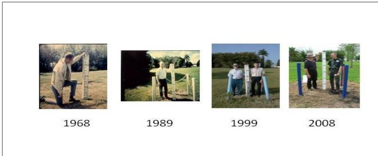
Figure 1. Decreases in soil depth since 1924 can be observed using the EREC subsidence post near Belle Glade, FL.
